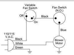
Figure 29 - Blower Wiring Diagram for Thermostat-Controlled Models
